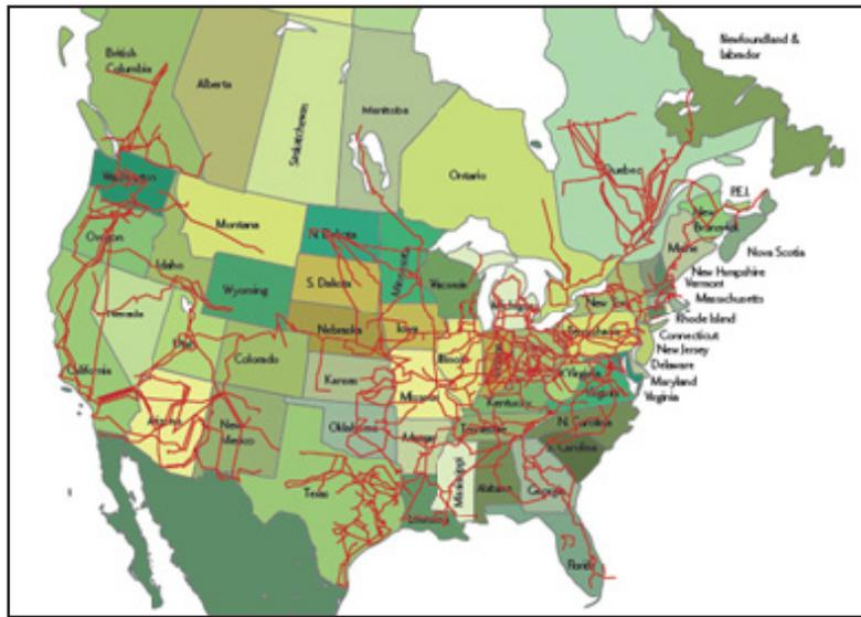
Figure 11) North American Electricity Transmission Lines > 500kV
